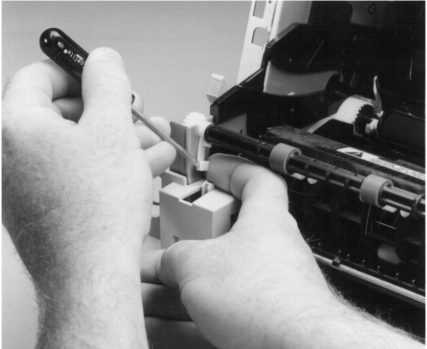
Figure 39. Exit roller removal
